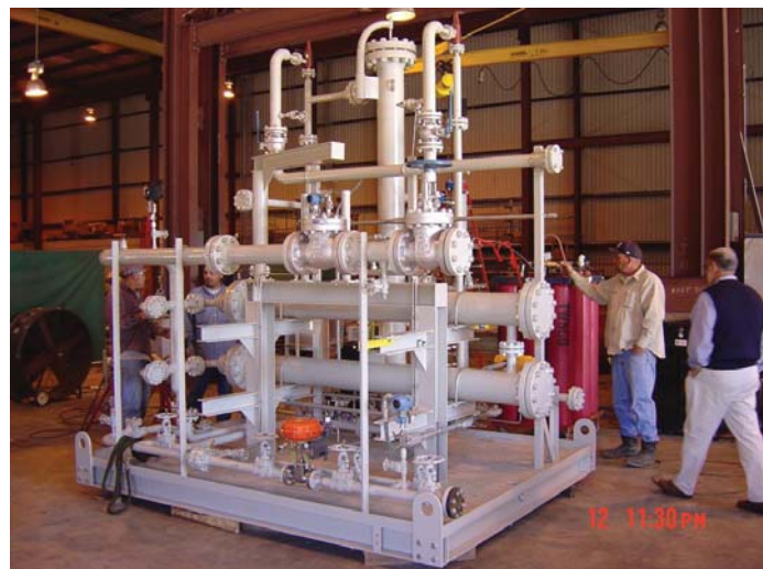
Compact membrane units are ideal for offshore installation.
