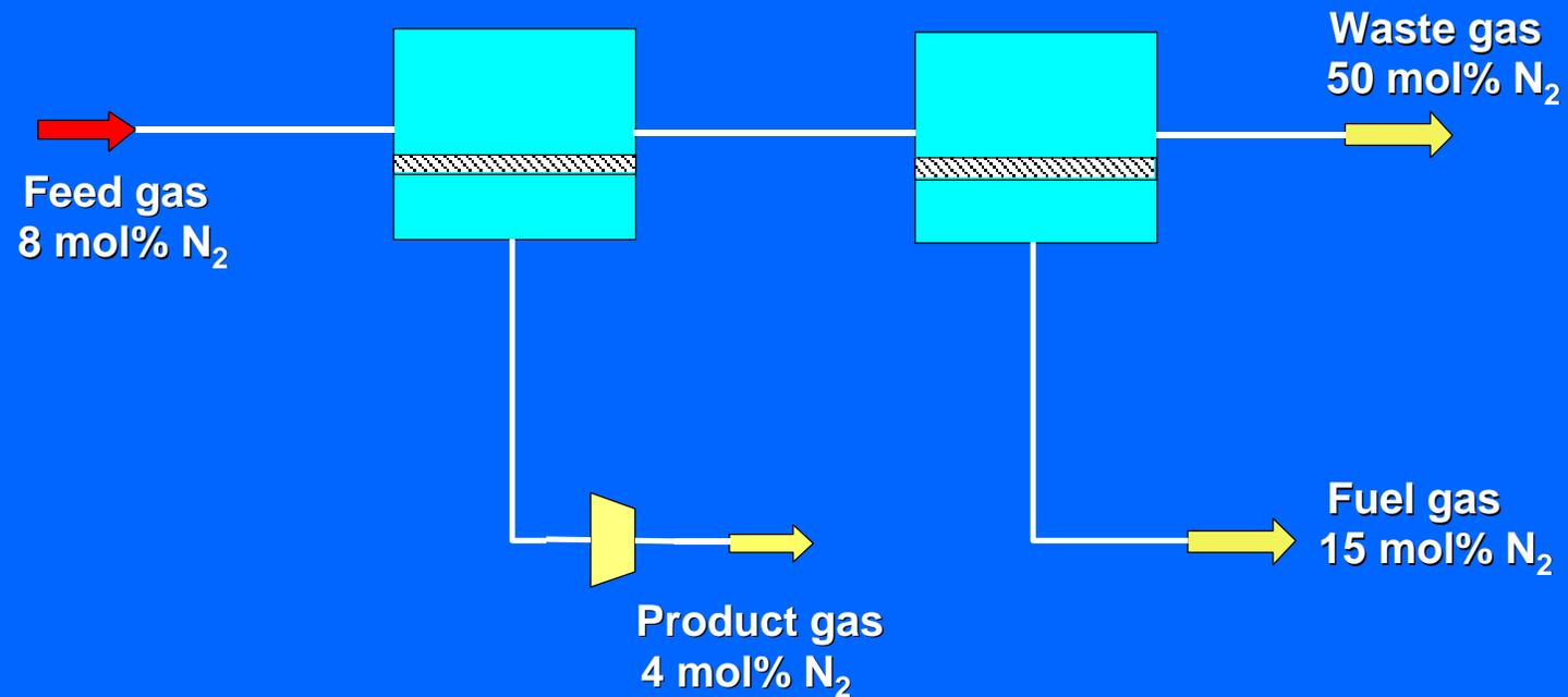
Two step process produces pipeline quality gas and fuel gas for process use.
