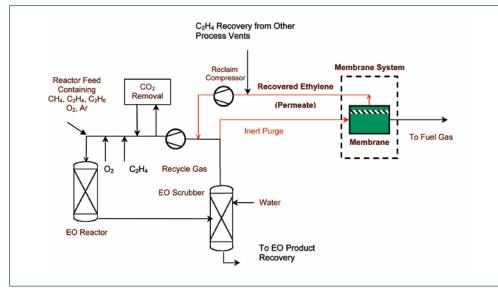
Figure 3. Schematic of EO plant ERU.
