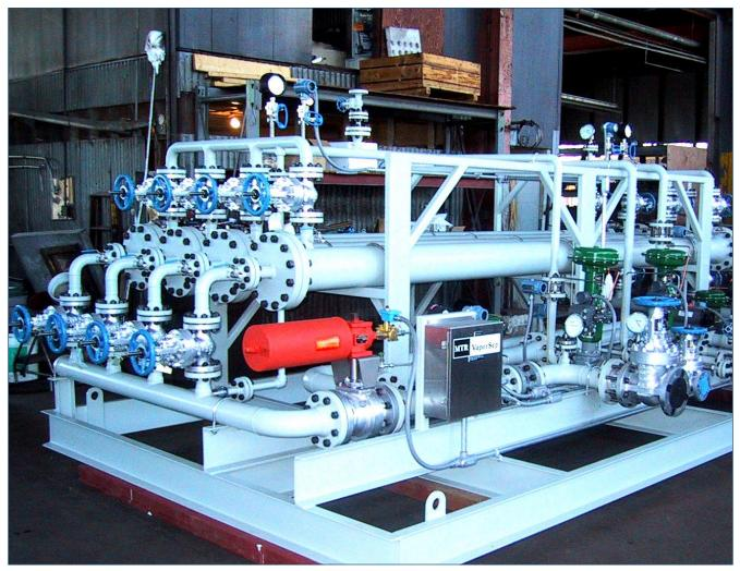
Figure 4. An ethylene recovery unit.
