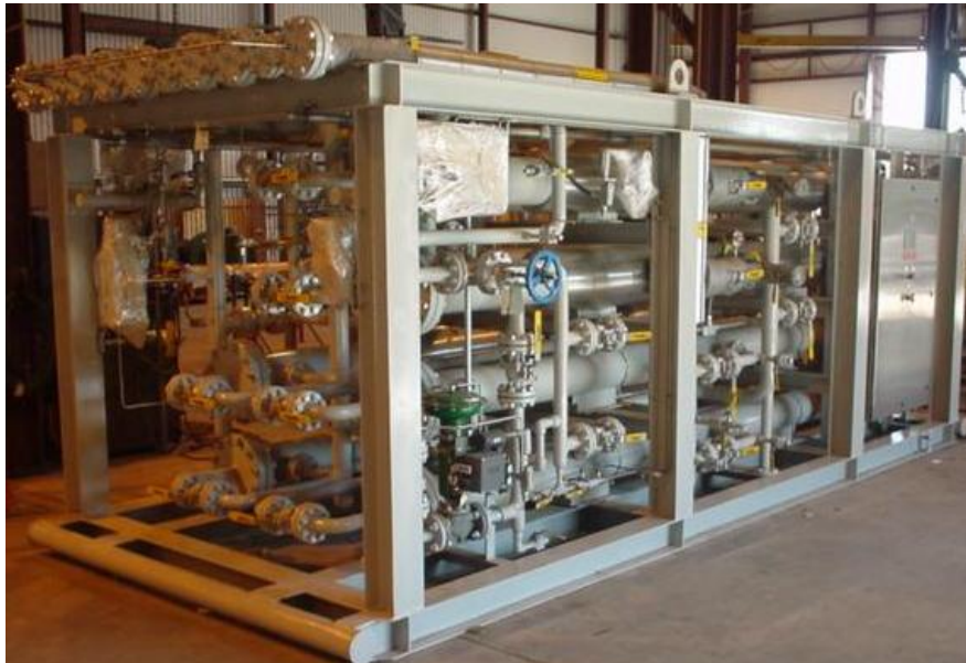
Figure 6. A skid-mounted mounted nitrogen-removal unit. The unit will process 1 MMSCFD of gas.
