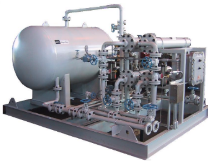
Figure 5. System Photograph of Unit installed in Omaha, Nebraska, reducing 6.5 mol-% N 2 in Natural gas to 2.5 mol-%.
