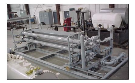
**Figure 5.** Photograph of FGCU designed to treat high hydrogen sulfide-content gas. Skid mounted with four horizontal pressure vessels shown in the photograph.
