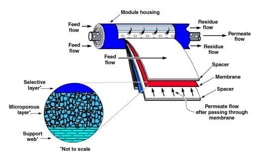
**Figure 1.** Schematic illustrations of a composite membrane and a spiral-wound module of the type used in fuel gas conditioning units.
