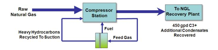
**Figure 3.** Block diagram of a membrane unit installed at a compressor station with a downstream NGL Recovery Plant.
